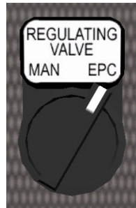
Fig. 28. Regulating valve switch
