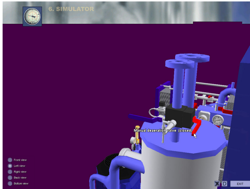
Fig. 16. Left view - Automatic and manual deaeration arrangement
