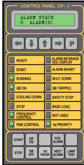
Fig. 15 Control panel - front layout
