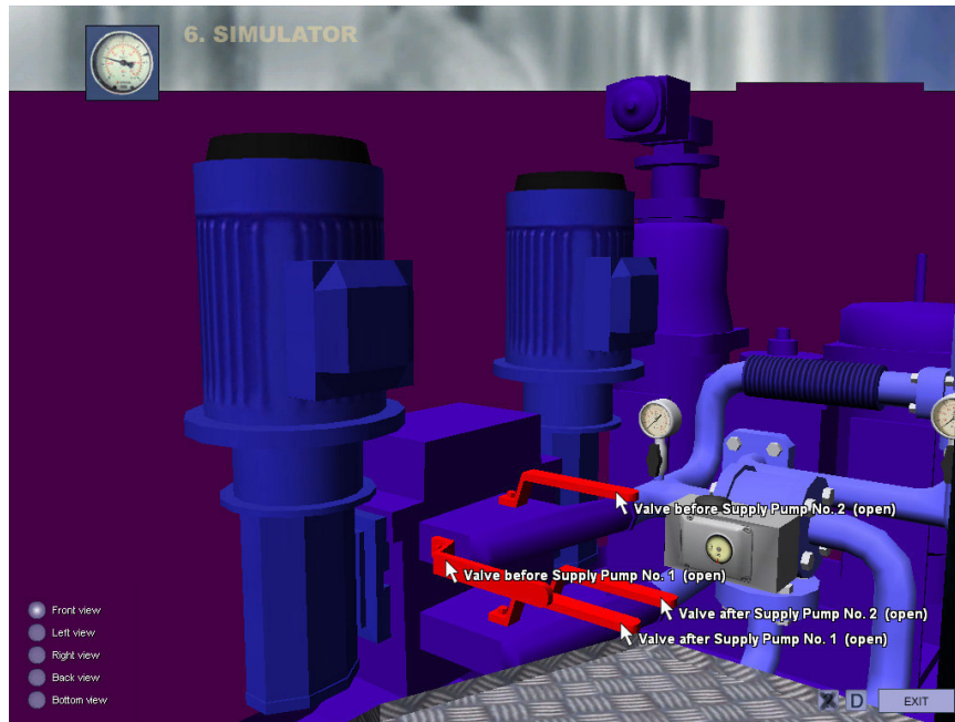
Fig. 14. Front view - Supply pumps with valves
