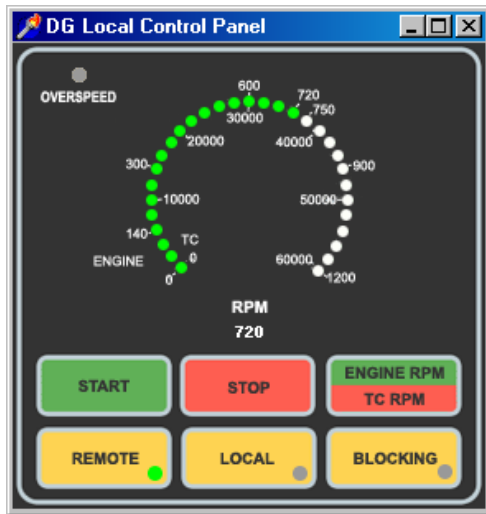
Fig. 13 Diesel engine local control panel
