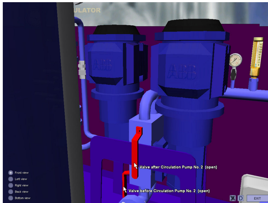
Fig. 17. Front view - Circulating pumps with valves
